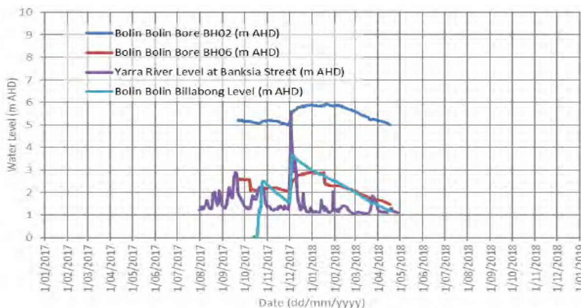
Figure 4-2 Surface water and groundwater levels as indicated in Figure 6- 9 of EES Technical Report N
