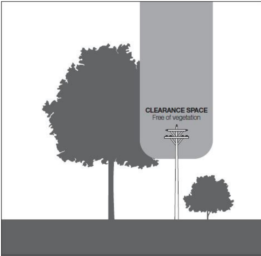
Figure 5: Clearance space for uninsulated low voltage and high voltage electric line (other than a 66 000-volt electric line) in hazardous bushfire risk area
