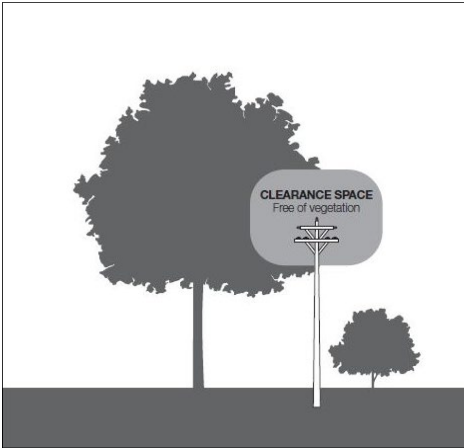
Figure 3: Clearance space for uninsulated high voltage electric line (other than a 66 000 volt electric line) in a low bushfire risk area
