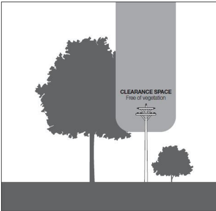
Figure 4: Clearance space for uninsulated 66 000 volt electric line in a low bushfire risk area
