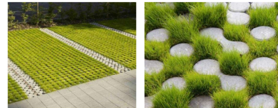
Potential permeable surface treatments
